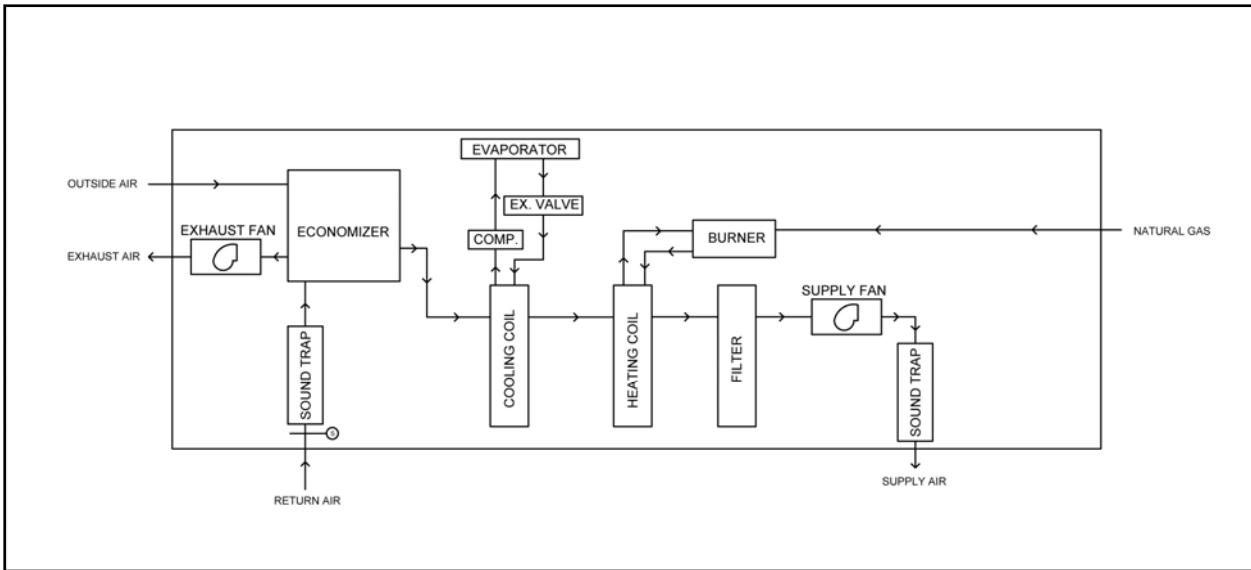
FIGURE 2 – RTU Schematic
