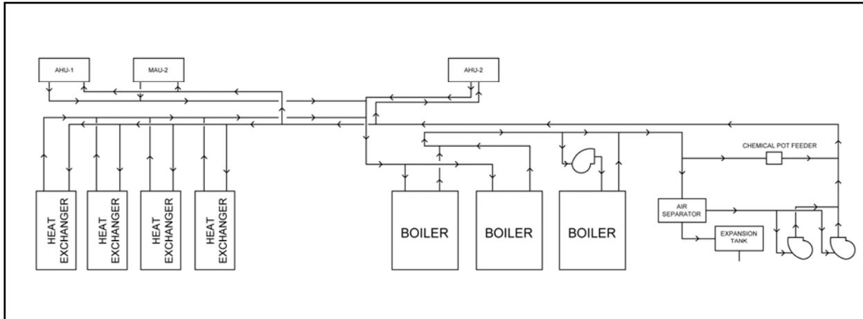
FIGURE 3 – How Water Schematic
