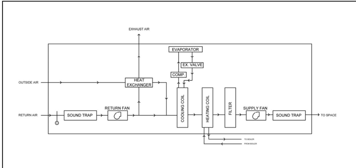
FIGURE 1 – AHU Schematic
