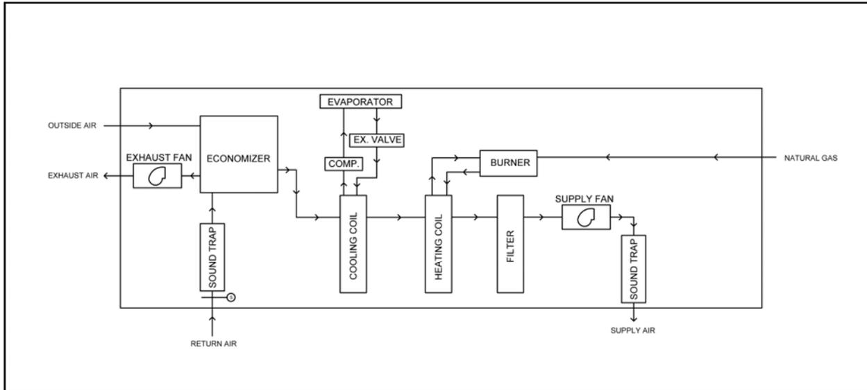
FIGURE 2 – RTU Schematic
