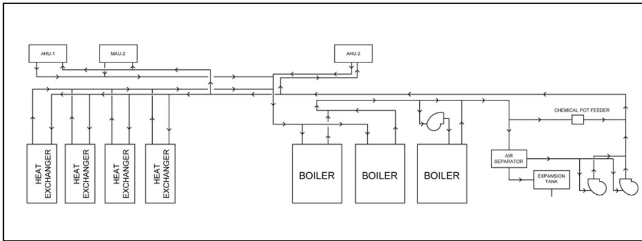
FIGURE 3 – How Water Schematic
