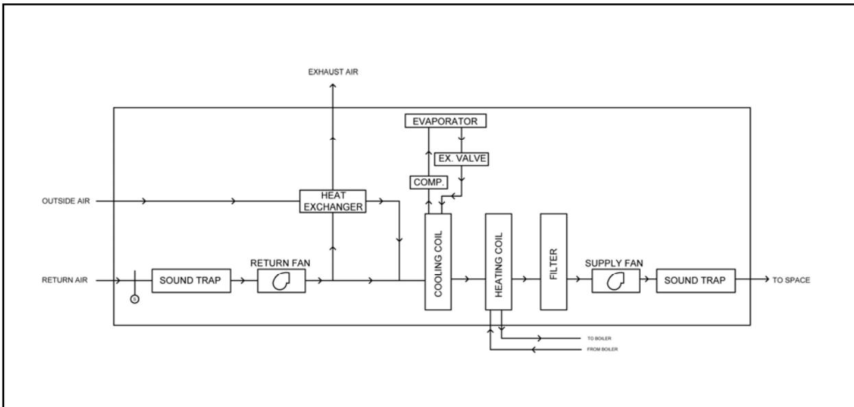
FIGURE 1 – AHU Schematic
